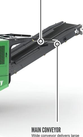
Wide conveyor delivers large stockpile capacity. Conveyor lowers and raises hydraulically.
