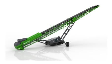
The 22.5 degree maximum conveyor angle allows for the highest stockpiles per conveyor length in the industry. With its durable truss frame, large feed hopper and base production capacity of 500 TPH with optional upgrades to 800 TPH, the McCloskey ST80T Stacker stands up well above the competition.
