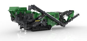
The combination of the Jaw Crusher along with the High Energy Screenbox and a recirculating conveyor deliver maximum productivity. The radial recirculating conveyor allows operators to either return material through the crusher jaws or to stockpile a separate finished product.
