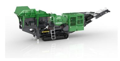
At 2.5 metres wide, the J40 jaw crusher is ideal for applications that require a high degree of mobility.
