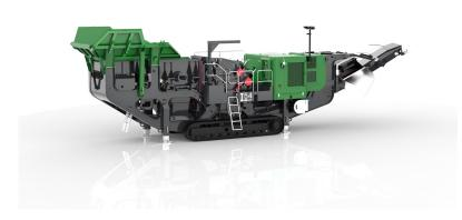
Available with various blow bar material options, the I54 is versatile and easily transported. It has a minimal setup time with integrated hydraulic folding hopper and stockpiling conveyors, maximizing on-site production time. The I54's versatility and upgraded design makes it ideal for some of the toughest applications worldwide, including asphalt recycling, concrete recycling, rock crushing, construction and demolition.
