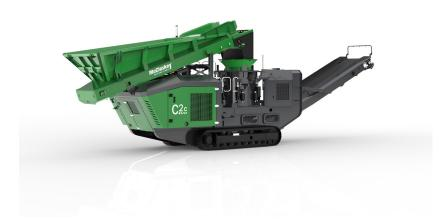
The McCloskey C2C Cone Crusher is the ideal portable secondary crushing solution for operators requiring high production rates in a compact footprint. Its unrestricted feed opening improves material feed intake and reduces the risk of blockage. The direct drive cone on the C2C has a minimum setting of 13mm (0.5") and a maximum feed of 185mm (7.28"). The variable speed of the crusher delivers the best combination of production and product shape, maximizing its efficiency in crushing.
