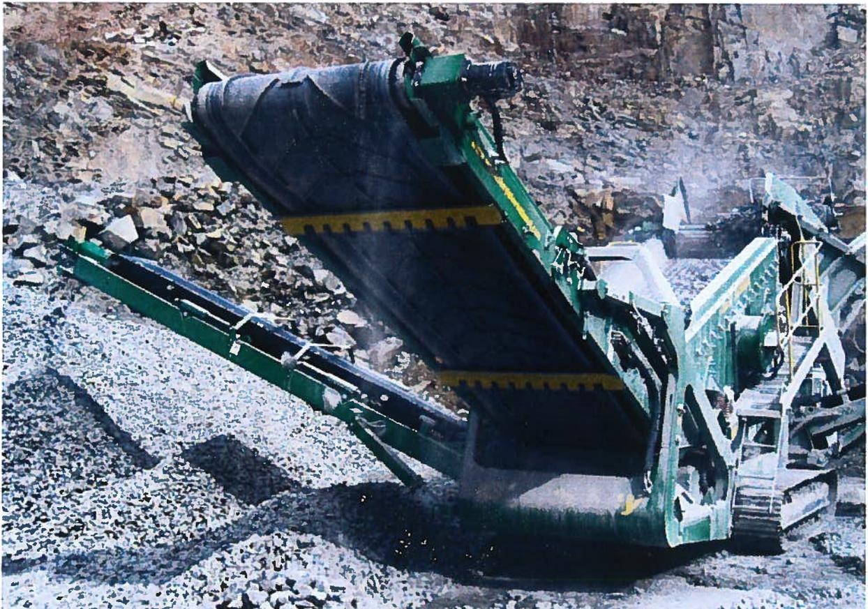
The R155 is able to handle larger material thanks to an open feed design that allows for free flow of material and high volume capacity.
