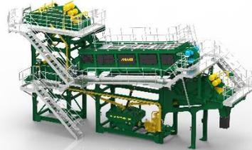
The log shafts rotate in opposite directions and are timed to obtain an overlap of the paddle shoes for maximum scrubbing action.
