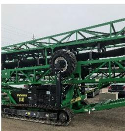
The ST80T Radial's unique tool free transport design allows the equipment to move freely from site to site without needing to remove the wheels, delivering true portability for multi-site projects and operations.
