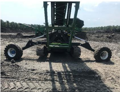
Built-in levelling indicators allow operators to position the stacker regardless of the ground evenness, with independent hydraulic jack legs to stabilize once in place. A level gauge allows operators to position the stacker for maximum production. The tires on the ST80T Radial have an aggressive tread pattern for better traction in rough terrain.
